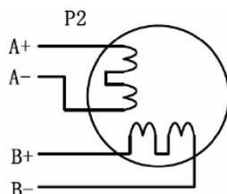
Figure 5: 4-lead Motor Connections
